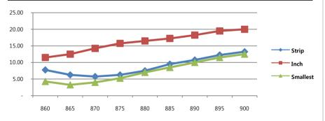
•STRIP reads up to 2.0 meters on metal, 20% shorter than SMALLEST, but double of INCH. It is recognized best performing among 6mm slim UHF metal tags.
