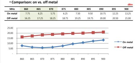
•STRIP reads 80% shorter off metal (or on non metal surface). It can be applied, therefore, only for metal application. For non metal application, please use SMALLEST NM.
