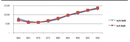
•STRIP reads almost same, regardless of whether it is fastened with metal bolt in two holes (located on both ends) or not. Stainless steel M3 bolt with round head is best fit for STRIP.
